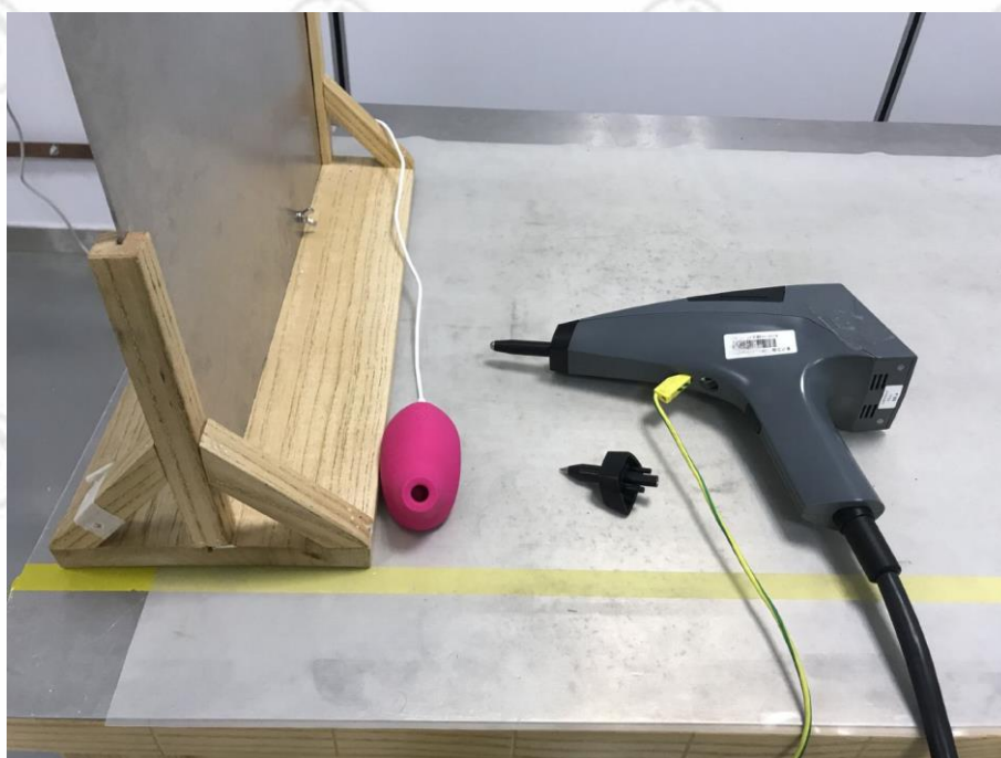
ELECTROSTATIC DISCHARGE TEST SETUP (CHARGING MODE)
